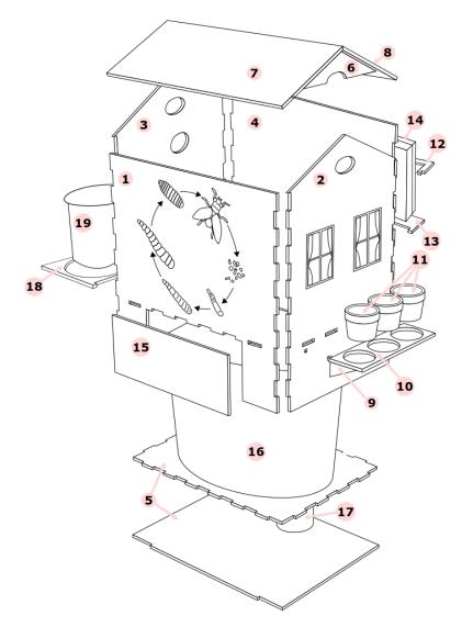
Figure 1. Exploded view of the rearing system for black soldier fly larvae.
