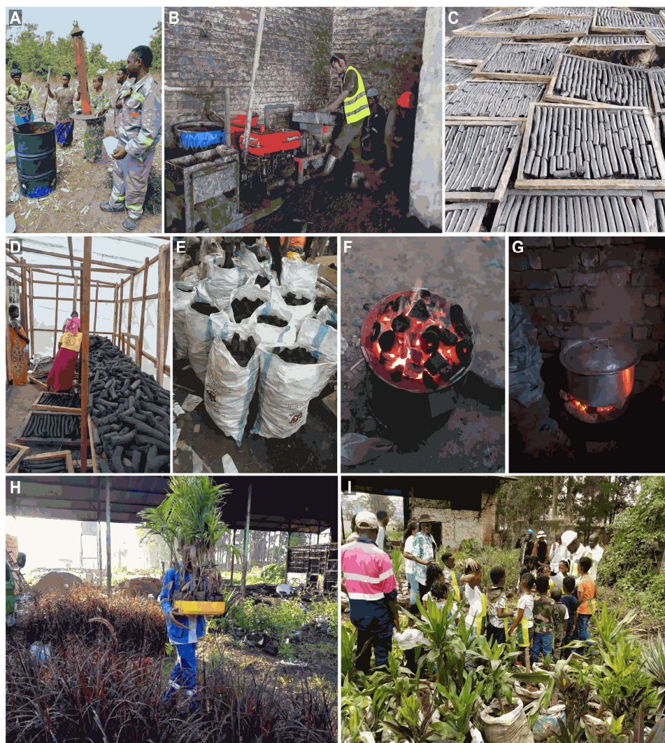
Figure 5. Panel of images related to biochar. (a) Workers operating a carbonizer modified from an oil drum; (b) Workers are operating the compaction-extruder; (c) briquettes are formed and laid out to dry; (d) workers stockpile dried briquettes; (e) briquettes are sold in bags, (f) smokeless flames generated by briquettes, (g)
